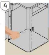
Use a spanner or socket to tighten the bolts and their washers.
